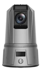
This portable outdoor network PTZ camera is an unique 4G wireless camera for rapid deployment of high definition video. With built-in 4G LTE wireless module and industrial lithium battery, the camera can be working in almost any places without the limitation of wired network and power input. This camera can be put on desktop, vehicle top, or stick to any metal surface thanks to the magnet base design of camera bottom.
