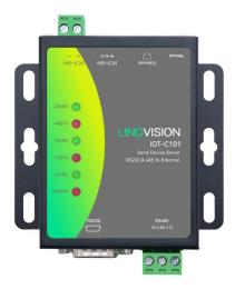
IOT-C101 is a multi-functional serial-to-Ethernet module that enables bidirectional transparent data transmission between Ethernet port and serial ports. IOT-C101 is a dual serial port server, using the Cortex-M7 solution, the main frequency is up to 400MHz, with stronger performance, faster transmission speed and higher reliability. It comes with 1\*RS232 and 1\*RS485 serial ports, and the two serial ports can work simultaneously.
