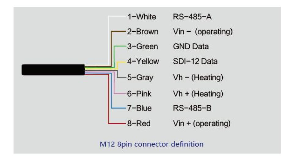
The device adopts an M12 8-pin connector, the different colored pins provide power and data
