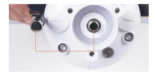
Plugin the cable and tighten it clockwise
