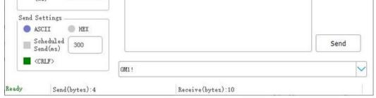
Then send "Read measurement value command 0D0!" to get the 6 measured values of this measurement, which are minimum wind direction 345.9 degrees, maximum wind direction 347.5 degrees, average wind direction 346.3 degrees, minimum wind speed 2.8m/s, and maximum wind speed 2.8m. /s, average wind speed 2.8m/s.
