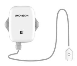
IOT-S500WD is a compact spot leakage detection sensor for detecting presence of water (or other liquids) and transmitting alarm using LoRaWAN® technology. With this low power consumption technology, IOT-S500WD can work up to 5 years with 4000 mAh battery. Combining with Linovision LoRaWAN® gateway and Linovision IoT Cloud solution, users can manage all sensor data remotely and visually and receive alarms via mobile APP.
