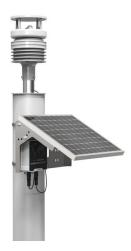
IoT Weather Station (IOT-S500WS5) is an all-in-one LoRaWAN® weather monitoring system for various atmospheric conditions, such as temperature, humidity, wind speed, wind direction, barometric and pressure. Consisting of 3 main parts, S500 Sensors, S500 Hub and solar panel, IoT Weather Station is designed to withstand the most challenging weather conditions and is easy to install in different scenarios to be widely used in meteorology, smart agriculture, smart building, etc.
