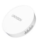
IOT-G63 is a 8-channel lightweight indoor LoRaWAN<sup>®</sup> gateway. Adopting SX1302 LoRa chip and high-performance CPU, IOT-G63 supports connection with more than 2000 nodes and can cover 15 km in sight and about 2km in urbanized environment. With compact size, it is ideally suited for offices, parking lots, campuses, hotels, exhibition centers and many other indoor areas. It also applies to provide coverage for indoor blind spots.
