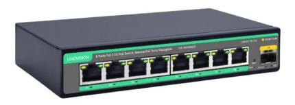
The POE-SWR308G25 provides 8\*10/100/1000/2500Mbps adaptive RJ45 ports and 1\*10Gbps SFP+ fiber module expansion slot. Each RJ45 port supports MDI/MDIX auto-flip and wire-speed forwarding functions. Ports 1 to 8 of them have PoE power supply function and support IEEE802.3af/at standard, which can be used as Power over Ethernet device and can automatically detect and identify the powered devices that meet the standard and supply power to them through the network cable.
