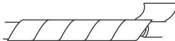
Figure 2.4.3 Third step during wiring – wrapping of insulation layers
